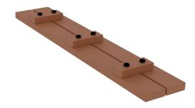
Please note that the support bars are flush with the side of plank A.
